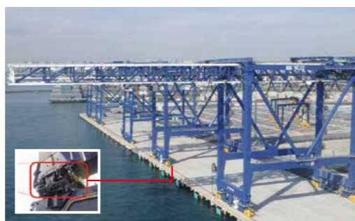
Adoption of a crane with seismic isolation functions capable of withstanding a major earthquake
